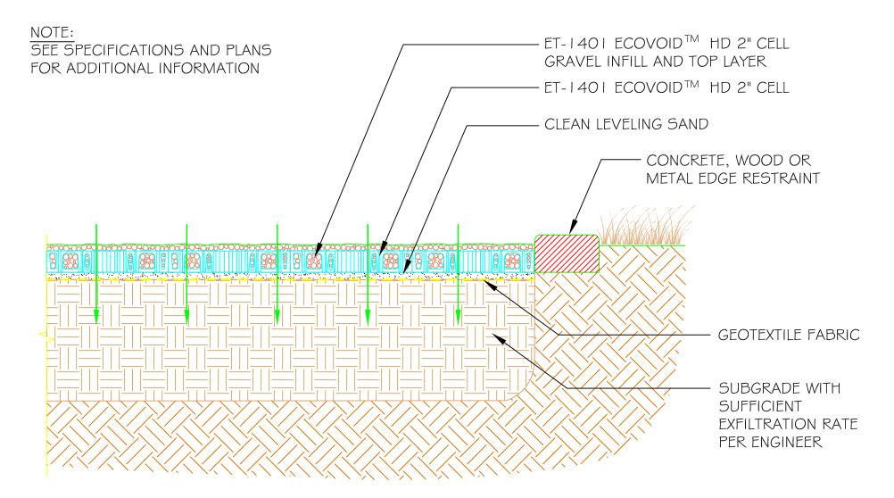
CONCEPT ECOVOID™ HD 2" CELL GRAVEL PAVER ON SUBGRADE INSTALLATION SECTION – FULL EXFILTRATION
